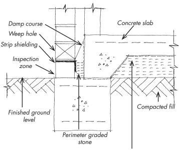
Under floor graded stone fill treatment (minimum compacted depth 75mm). Alternatively the underfloor graded stone can be omitted and the penetrations through the slab protected by an approved system
