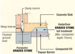
Graded stone barriers incorporate carefully graded and shaped, high quality granite particles which can be placed in a layer under the entire concrete slab area, around the base of stumps in an elevated building, as a partial barrier around the perimeter of the building or around individual penetrations (combinations of physical and chemical barriers may be necessary in some instances).
