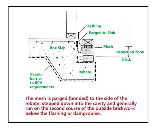
Stainless steel mesh barriers incorporate finely woven, marine grade stainless steel mesh which can be used in the same manner as the traditional ant cap, placed under the entire concrete slab area, as a partial barrier around the perimeter of the building or around individual penetrations (combinations of physical and chemical barriers may be necessary in some instances).
