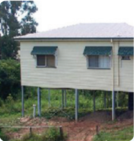
Do not build underneath a property or over easements unless all regulations are met. Interfering with the natural flow of water, particularly on a sloped allotment could cause flooding. Photo (right) courtesy of The Courier-Mail.
