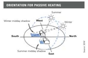
**Orientation for passive heating** is about using the sun as a source of free home heating. Put simply, it involves letting winter sun in and keeping unwanted summer sun out. This can be done with relative ease on northern elevations by using shading devices to exclude high angle summer sun and admit low angle winter sun. [See: Shading]
