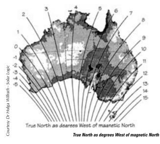
Note that solar north deviates significantly from magnetic north throughout Australia and should be taken into account when orienting a home. All references to north in this guide are to solar north not magnetic north.
