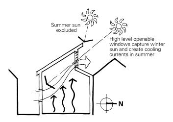
**On sites with poor orientation** or limited solar access due to other constraints, an energy efficient home is still achievable through careful design. A larger budget may be required. Use of advanced glazing systems and shading can achieve net winter solar gains from windows facing almost any direction while limiting summer heat gain to a manageable level. [See: Passive Solar Heating; Glazing; Shading]
