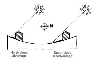
**A north facing slope** increases the potential for access to northern sun and is ideal for higher housing densities. A south facing slope increases the potential for overshadowing.
