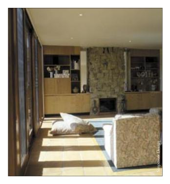
**'Solar access'** is the term used to describe the amount of useful sunshine reaching the living spaces of a home. The desired amount of solar access varies with climate.
