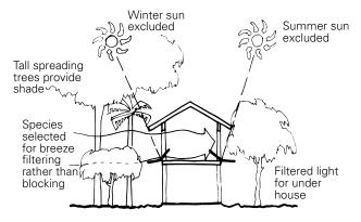
**Choose** or design a home with maximum exposure to cooling breezes and limited or no exposure to direct sun (depending on climate). Use careful design to improve performance in the case of poorly oriented sites or existing homes. [See: Passive Cooling]
