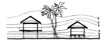
**Design** narrow, elongated building forms for best performance, with the long elevations opening up to cooling breezes. Elevating the house so that air can circulate beneath it will also assist performance.
