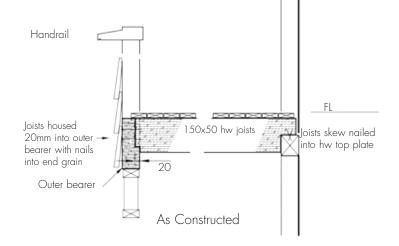
Cross-section of Ascot deck as constructed.
