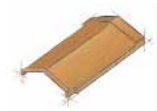
Vee Ridge (130°) Dimensions: 430L x 265W x 88D Cover length: 400
