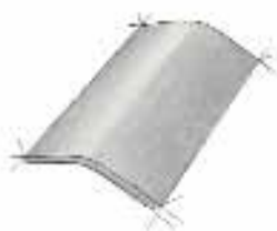
Standard Ridge (130°) Dimensions: 430L x 250W x 85D Cover length: 400
