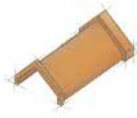
Steep Pitch Vee Ridge (81°) For roofs over 45° in pitch Dimensions: 430L x 265W x 185D Cover length: 400
