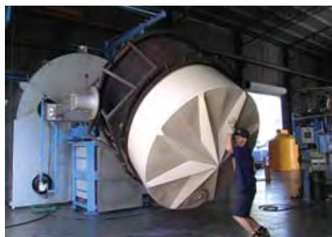
The birth of a polyethelene rainwater tank as it exits the mould.
